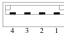
USB Connector pinout front view
